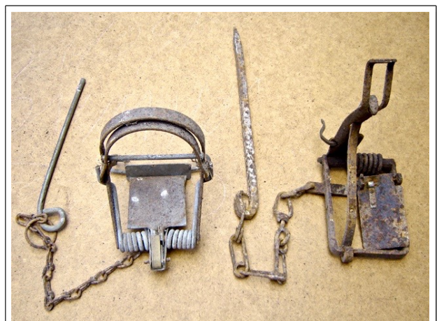
Fenn trap (left) and Sawyer trap were brought in as hopefully more humane than the gin trap.
